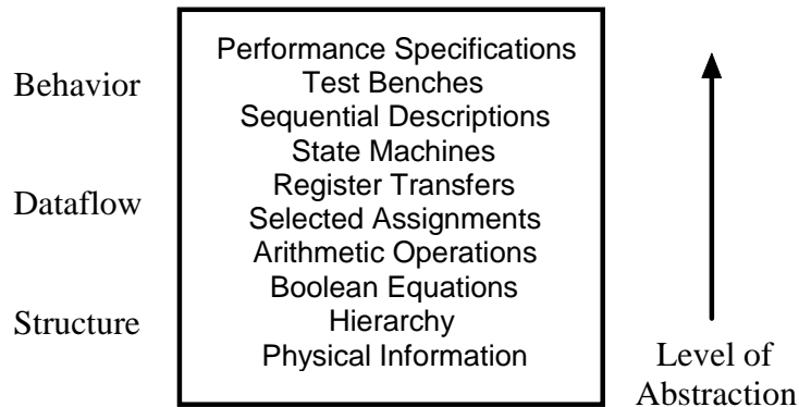
Figure 7-2: VHDL allows you to describe a system at many levels of abstraction.
